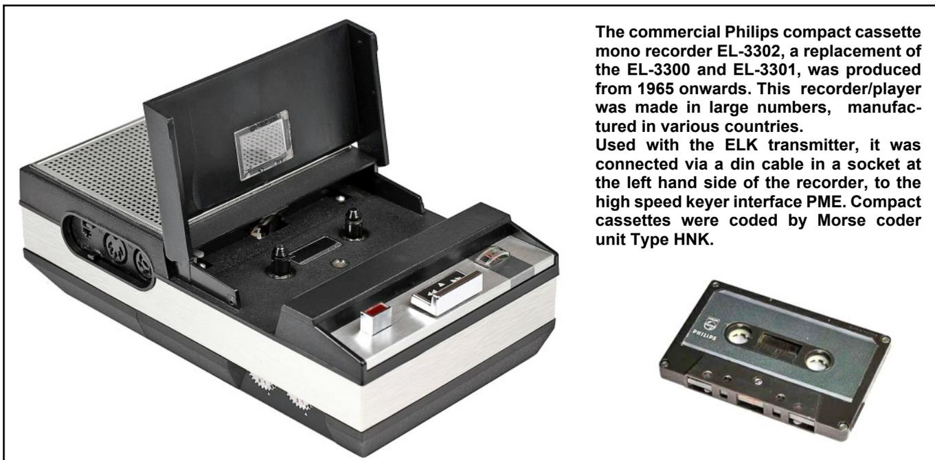
**The commercial Philips compact cassette mono recorder EL-3302, a replacement of the EL-3300 and EL-3301, was produced from 1965 onwards. This recorder/player was made in large numbers, manufactured in various countries.**
