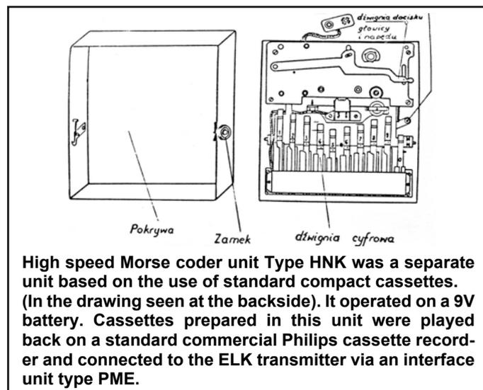
High speed Morse coder unit Type HNK was a separate unit based on the use of standard compact cassettes. (In the drawing seen at the backside). It operated on a 9V battery. Cassettes prepared in this unit were played back on a standard commercial Philips cassette recorder and connected to the ELK transmitter via an interface unit type PME.
